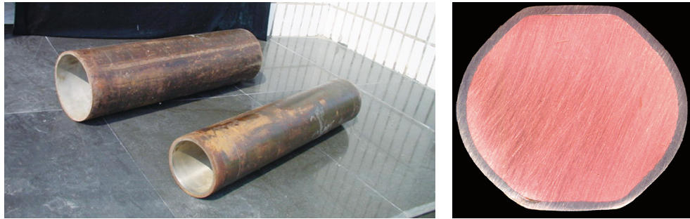
图7 爆炸焊接复合管材与棒材 Fig.7 Clad tube and bar by explosive welding
